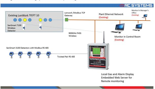
RC Systems first provided a free service to re-commission the old Lonwork detectors to make sure they were functioning properly, and then added a gateway to connect the Lonwork to the plants' existing Ethernet network.
